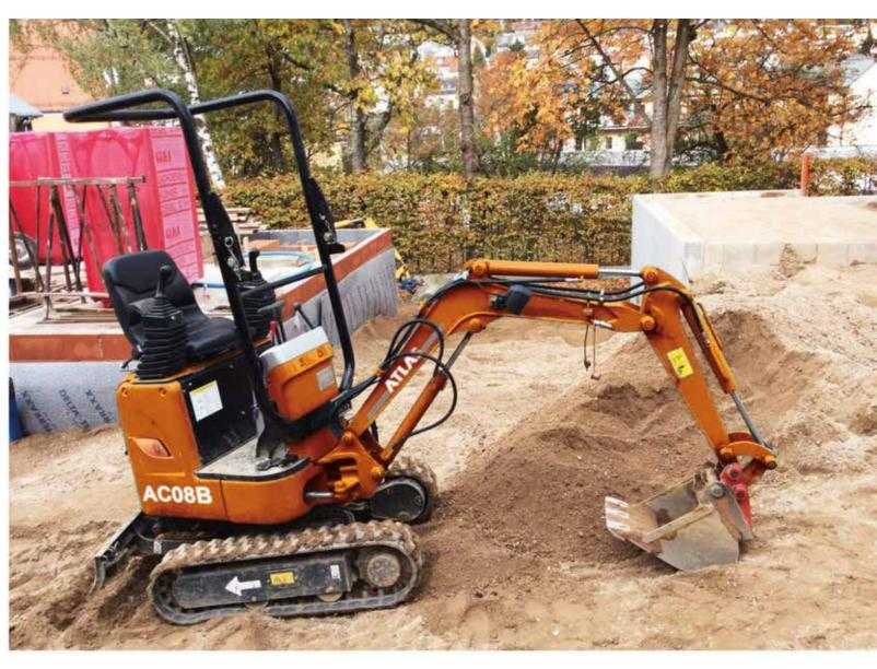
Engine netpower:7.2kW Machine weight:1010kg
