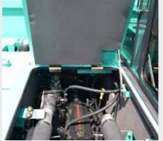
ENGINE CUMMINS QSB6.7 168 KW POWER.
