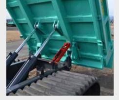
**DUMPING ANGLE** It has a maximum angle of 60° for the efficient unloading of materials.
