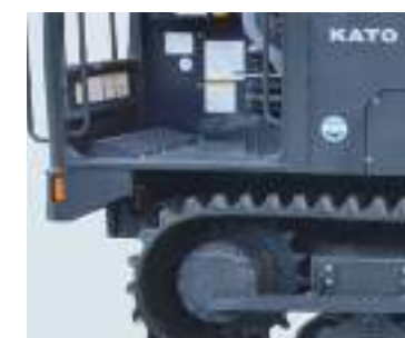
Flat foot space is for easy maintenance.
