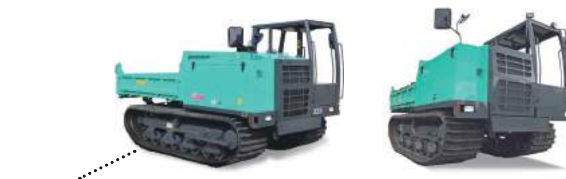
Maintenance parts are centralized on the right side.
