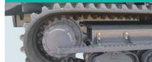
3 split sprockets can be replaced without removing the rubber shoe.
