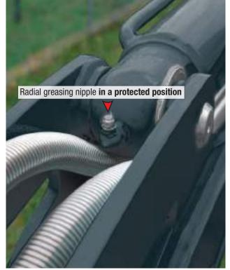
Protected and accessible greasing nipples
