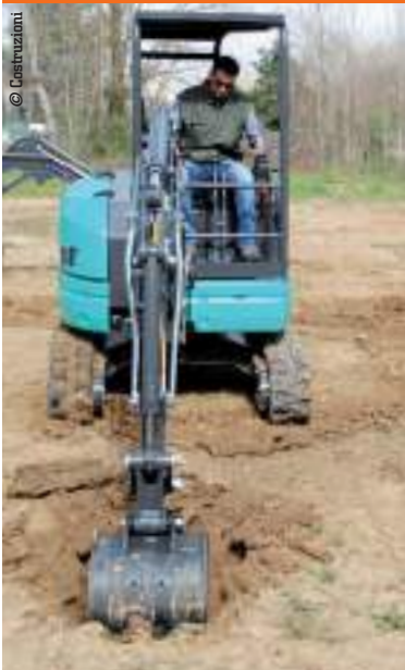
Offset boom Better visibility on digging operations
