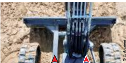
Offset boom Better visibility on digging operations
