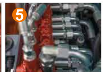
Main control valve
